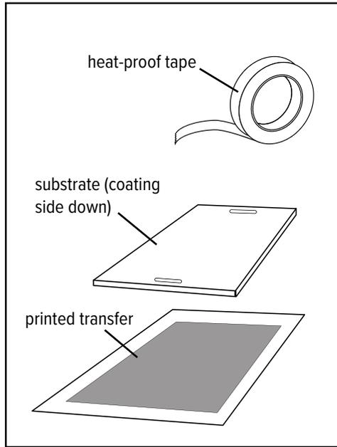
**Step 2:** Place substrate (coating side down) onto printed transfer sheet. Maintaining appropriate bleed for your substrate, use heat-proof tape to attach the substrate to the transfer sheet.
