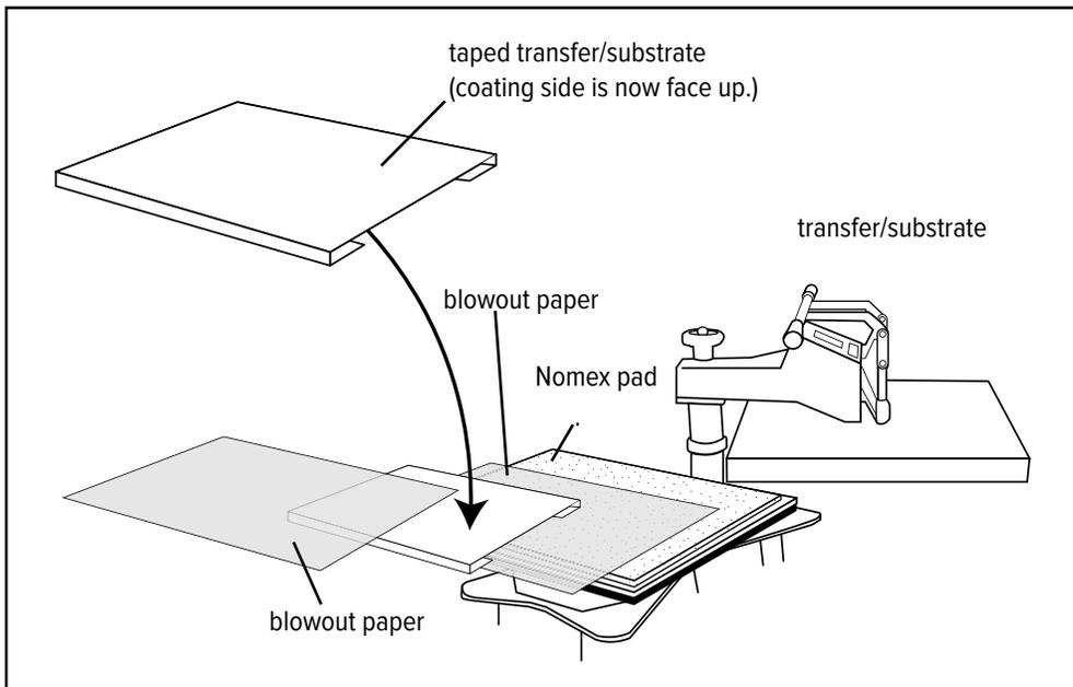
**Step 3:** Flip taped transfer/substrate (substrate coating will be face up at this point, but covered from view by the transfer paper) and place it in the heat press between the two layers of blowout paper.
