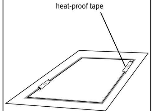
**For aluminum and other flat/thin substrates:** Substrate is taped flat to transfer.
