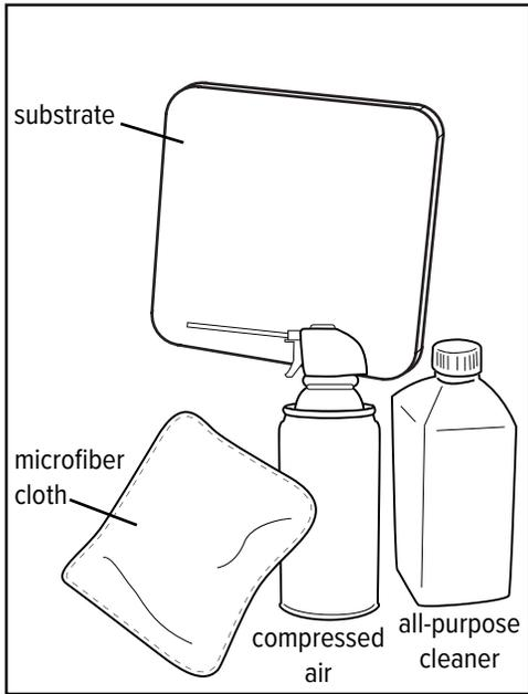
**Step 1:** Clean substrate using microfiber cloth, all-purpose cleaner, and/or compressed air.
